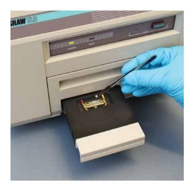
The Harshaw 3500 includes a sample drawer for a single element TLD dosimeter, a linear, programmable and precisely controlled heating system and a cooled photomultiplier tube to measure the TL light output.
